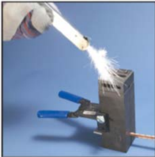
Igniting the accelerant
