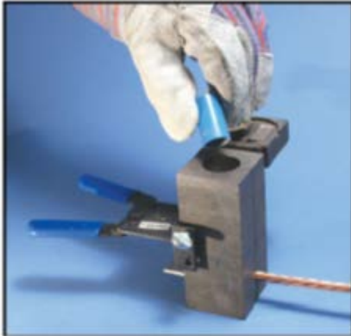
Pouring Weld metal powder into a mold
